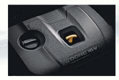
Nu 2.0 MPI gasoline engine Max. power 157 ps @ 6,200 rpm (EURO 2) Max. torque 20 kg·m @ 4,000 rpm (EURO 2)
