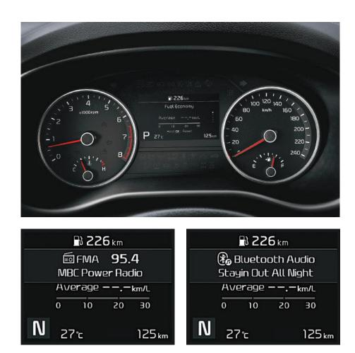
**3.5-inch monochrome TFT-LCD** Valuable information including total mileage, outside temperature, average speed and distance traveled is clearly displayed, enabling you to keep your eyes on the road ahead.
