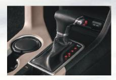
Automatic transmission This six-gear unit features auto shift lock to prevent any unintended acceleration from happening.
