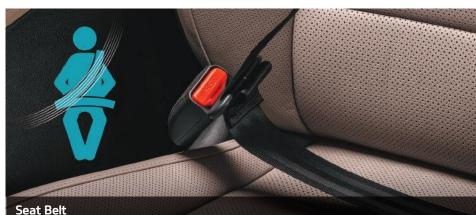
Seat belt pretensions pull the front-seat passengers with full force into the seat, in case of abrupt halts or collisions, preventing them from colliding against the dashboard and positioning them to receive maximum air bag protection.
