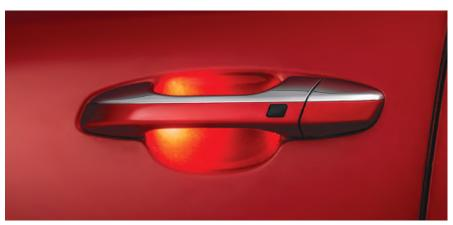
Smart welcome system Approach your vehicle with the smart key fob and the Sportage springs into life once you're comfortably within range. Welcome lights turn on and the outside mirrors unfold into position so that you're ready to be on the move again.
