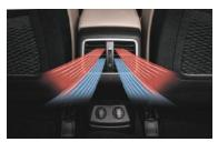
Ventilation and USB charger for 2nd row passengers Cold or warm air is available when needed and your rear seat passengers can also recharge their devices on the go.
