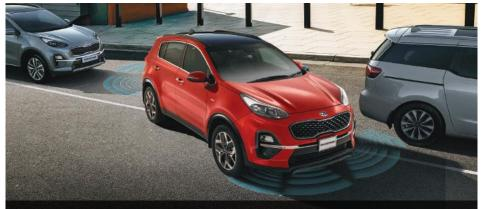
Parking Distance Warning-Forward (PDW-F) Ultrasonic sensors on the front and rear bumpers detect objects or pedestrians and let you know their distance from your vehicle.
