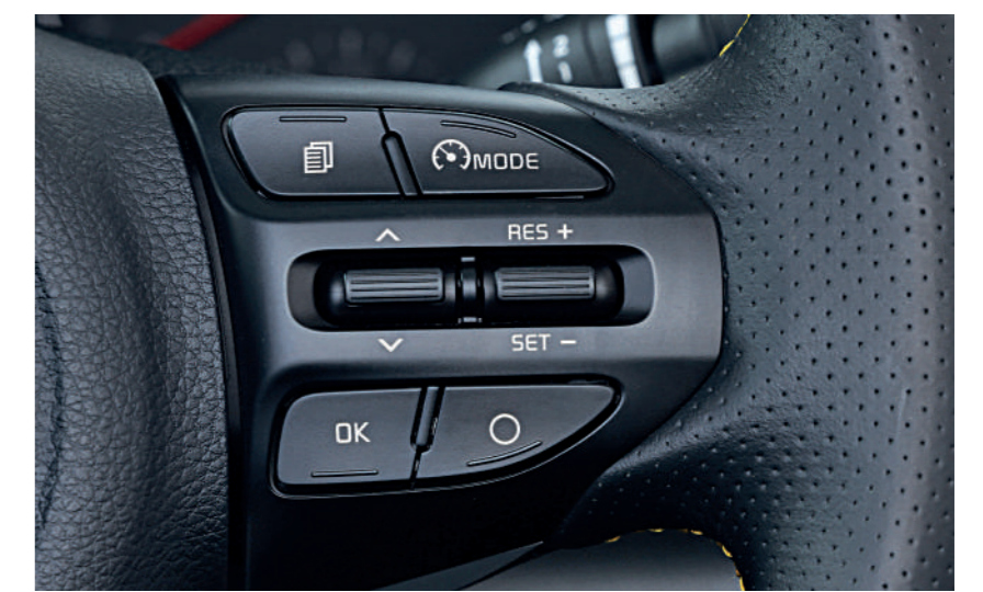
Cruise Control with Manual Speed Limit Assist Set and maintain a constant speed and simply step on the brake or accelerator when you want to disengage.
